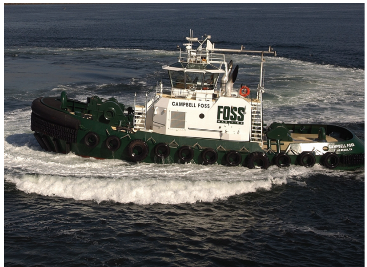
The Foss hybrid tug will look almost identical to its sister Dolphin-class tugboats, but will be quieter, cleaner and more fuel efficient, using hybrid technology.
